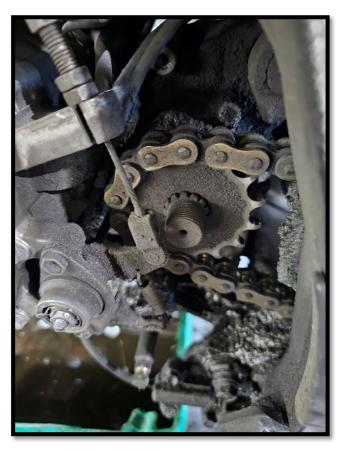
This motorcycle is missing the nut and lock washer that holds the front sprocket on. One very lucky customer that it didn't come off and break the cases.
